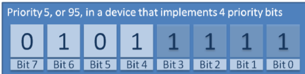
Figure 7.15 How a priority of binary 101 is stored by a Cortex-M microcontroller that implements four priority bits
